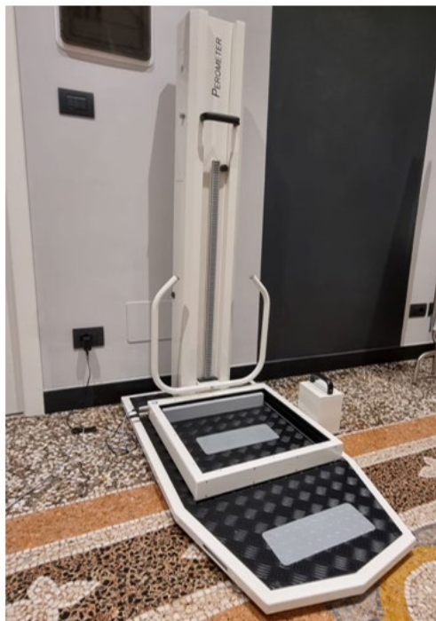
Fig. 1. Photograph of the opto-electric Perometer (400T model Pero-System).
