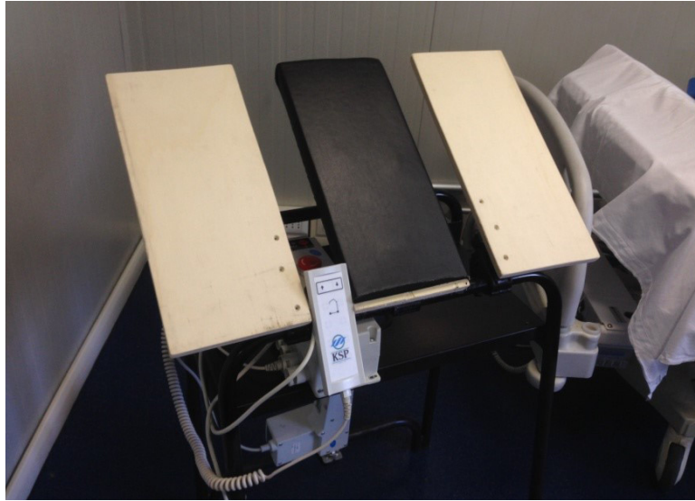
Fig. 2. Paddles for evaluation of proprioception. The central paddle is moved by electric controlled servomotor.
