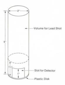
Fig. 1 Device for applying pressure to experimental site. Radioactive detector is placed in slot. Lead shot is inserted into chamber above to vary applied pressure
