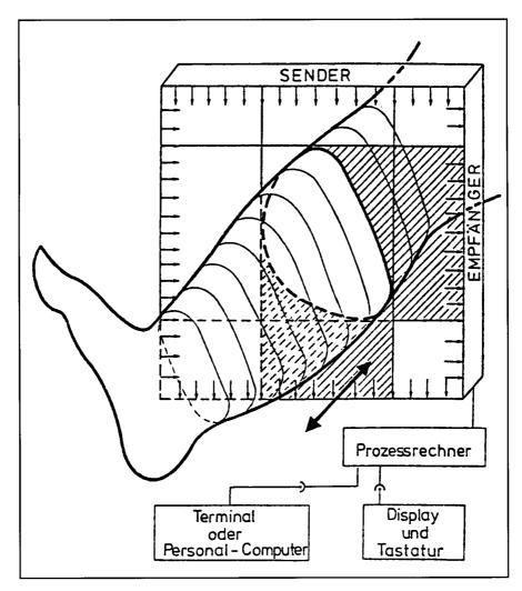
Fig. 2. Diagram of operation of the Perometer (reproduced with permission from Professor J-U Fischbach).
