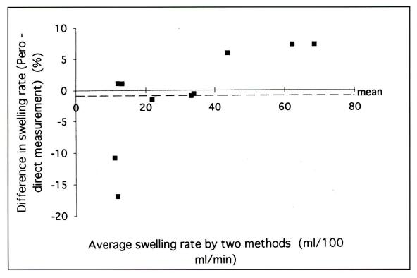
6b) Differences in apparent swelling rate obtained from the Perometer (Pero) and by direct measurement (i.e., tape measurement of circumferences) of the frustum, calculated as (Perometer minus direct measurement)/mean swelling rate x 100%, plotted against the average of the two methods. The mean difference (indicated by a dotted line) was  $-0.8 \pm 7.8\%$ , or (+)0.83  $\pm 2.37$  ml/100 ml/min.
