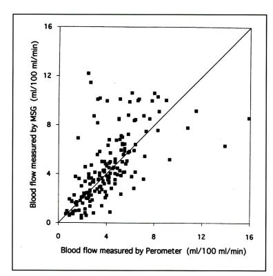
Fig. 8a) Scatter diagram of all the individual blood flow measurements (recordings with initial vertical slopes omitted) obtained from the arms of healthy subjects using venous occlusion plethysmography. The Perometer and the mercury strain gauge (MSG) have been compared. Considerable scatter is evident. The equation describing the regression line is y = $[0.75 \pm 0.07]x + [1.43 \pm 0.33]$  (mean  $\pm$ s.e.m.), r = 0.63, P << 0.0001, n = 174.
