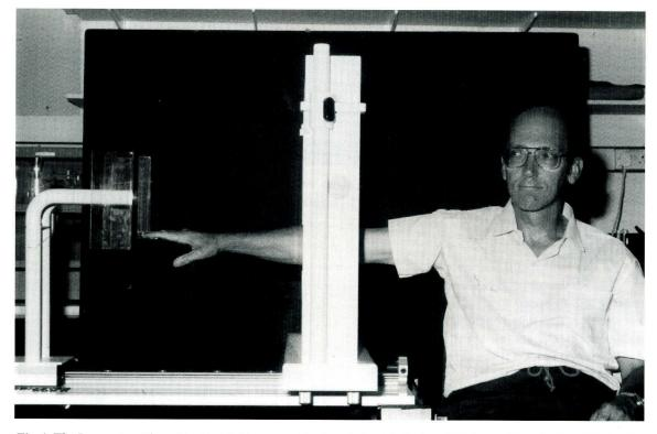
Fig. 1. The Perometer. The subject holds his arm out horizontally with the hand resting on the perspex support. The measuring frame is moved by hand along the length of the limb towards the shoulder and then back towards the wrist. The Perometer computes the volume from a large number of vertical and horizontal diameter measurements.
