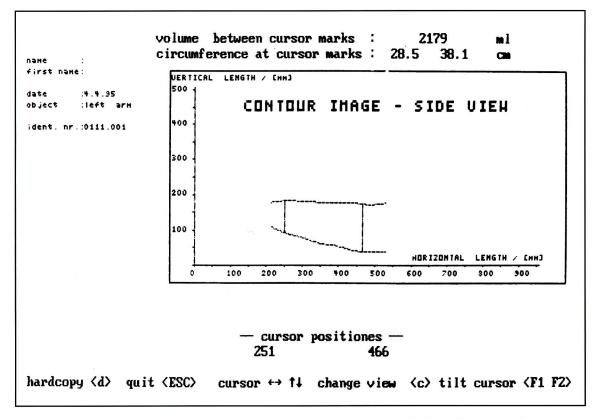
Fig. 4. Profile (side view) of a lymphedema arm generated by the Perometer. The circumferences at the two cursor positions and the volume of the enclosed segment are given. The hand cannot be accurately recorded, and is not shown.
