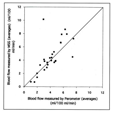
8b) Scatter diagram of average blood flow measurements (same subjects as in Fig. 7a) comparing the Perometer and the mercury strain gauge (MSG). The scatter of the results is less than in Fig. 7a. The regression equation is now  $y = [0.95 \pm 0.21]x + [0.61 \pm 0.92]$ (mean  $\pm$  s.e.m.), r = 0.68, P = 0.0001, n = 27.
