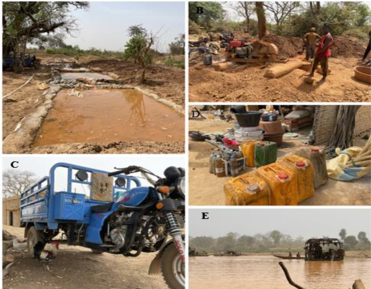
Figure 3: Some tools and processes used in artisanal gold mining (photos El. H. S. Top, 2022; G. Arnaud-Fassetta, 2023)/ A: Cyanidation catchments sluice; B: Spitter and washing workshop; C: Tricycle for transporting ores; D: A few objects used in artisanal gold mining on display at a market at a mining site on the banks of the Faleme; E: Artisanal dredgers in operation in the Faleme River.
