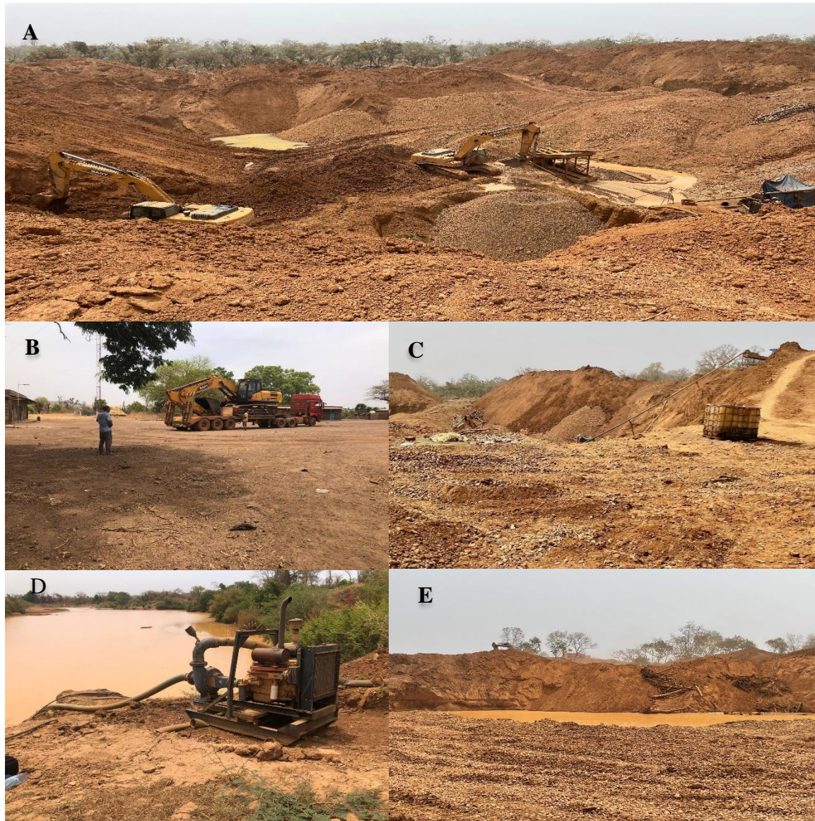
Figure 6: Equipment used in semi-mechanical mining by Chinese miners (photos G. Arnaud-Fassetta, 2023; El. H. S. Top, 2023) / A: Mechanical shovels in operation on a Chinese semi-mechanical trail; B: A Chinese operator takes delivery of a machine intended for gold mining; C: Lubricant tank and a sludge evacuator; D: Generator used to supply water to the gold processing site; E: A bene truck in operation on a semi-mechanical site.
