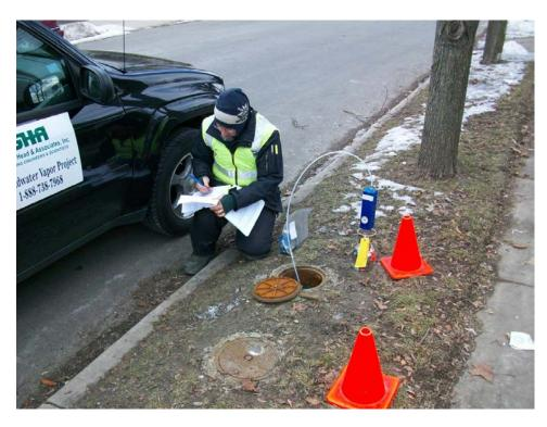
Figure 4: An expert measuring groundwater vapors in Endicott's TCE plume. Photo by author
