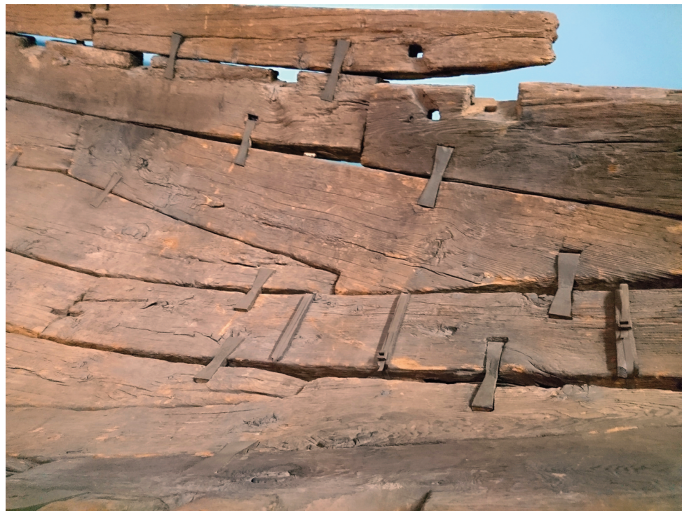
FIGURE 2: Detail of the plank joinings of the Carnegie boat (photograph: E. Peters, 2017) © Carnegie Museum of Natural History, Carnegie Institute, 2017.
