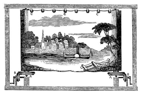
Figure 1: A panorama or moving tableau, showing its frame and mechanism, which would have been hidden from the audience. From *Scientific American* 4.13 (16 December 1848): 100.
