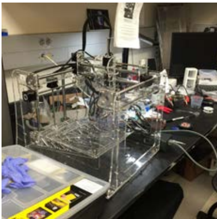
A Fab@Home Model 1 3D printer. It is an open source 3D printer project that provides instructions and parts for people to build their own 3D printers at home. Alice built that printer on her own, and with help from Divneet Mandair and Ned Premyodhin, is getting it to work.
