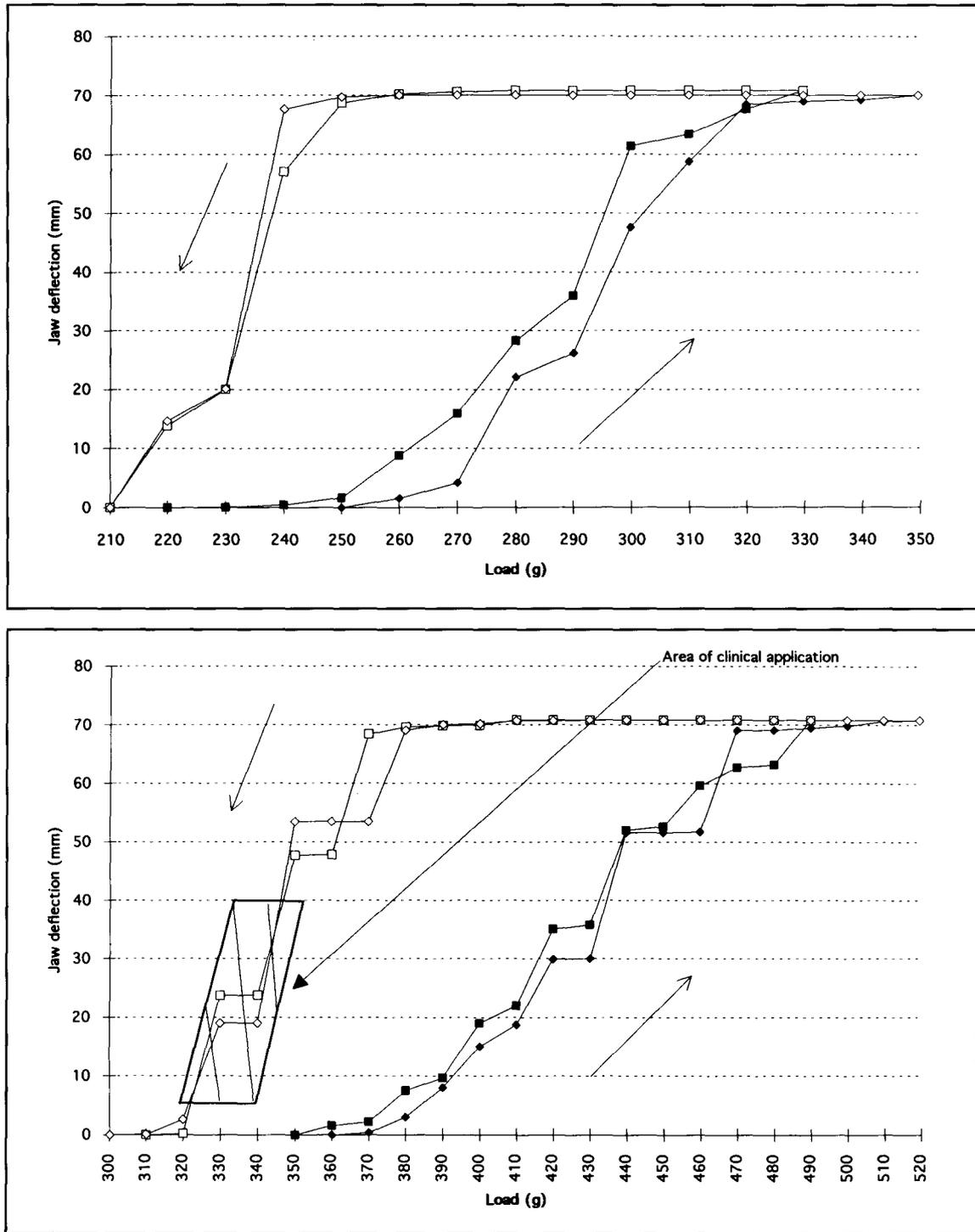
Fig. 3. Hysteresis curves produced by either rapid loading and removal (squares) or slow loading and removal (diamonds) for (a.) LE-029C-6, (b.) LE-031C-6.
