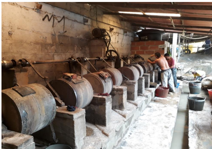
Figure 2: Workers operating ball mills ( cocos ) in artisanal gold processing facility. Visits to entables , Segovia, 11 May 2019. Photograph by author.
