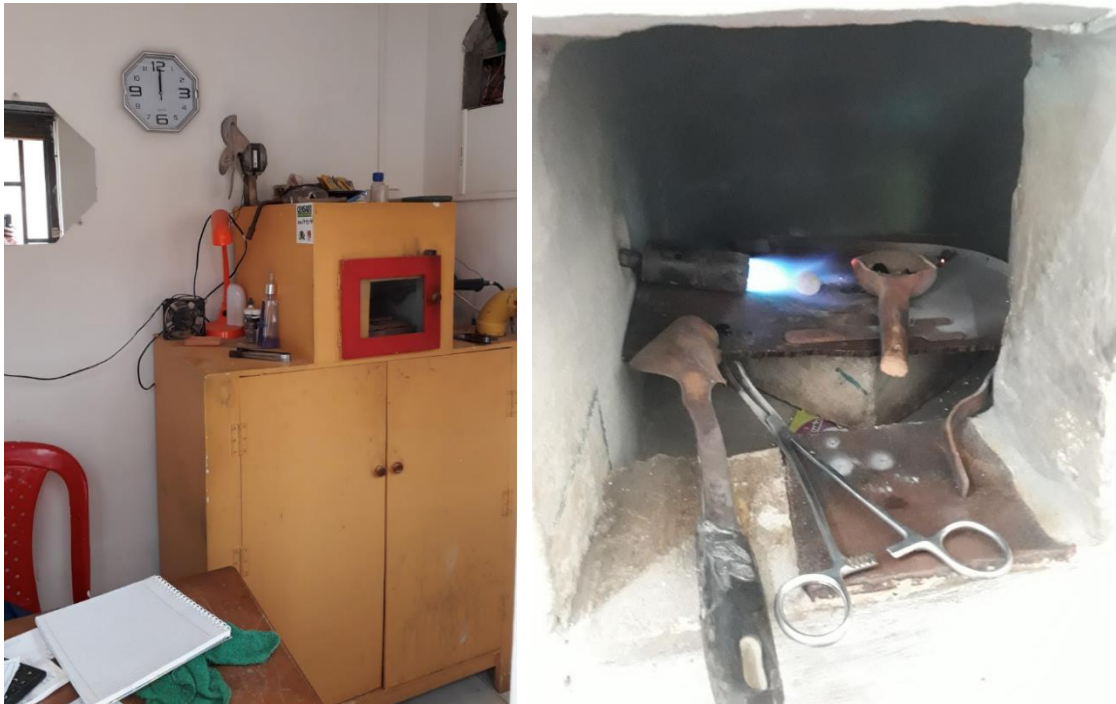
Figure 5 (left): Gold smelter for artisanally mined gold. Figure 6 (right): Amalgam burning in gold smelter for artisanally mined gold. Visits to gold smelting shops, Segovia, 11 May 2019. Photographs by Author.
