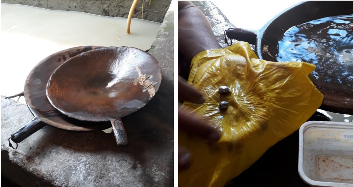
Figure 3 (left): Traditional gold pan (batea) used to recover the mercury amalgam in artisanal gold processing. Figure 4 (right): Worker recovering mercury amalgam by squeezing it through a cloth. Visits to entables, Segovia, 11 May 2019. Photographs by author.
